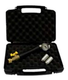
The Jet Nozzle VRI IPX 5/6 Set, is used for the verification test of the degree of protection to the risk of water penetration provided by the wrapper of equipment in fulfillment of IPX5 and IPX6 according to the IEC 60529 Section 14.2.5. & 14.2.6.
