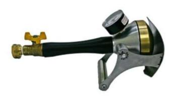
The VRI SW Spray Shover Tester IPX 3/4 is designed to perform tests in large and small scale products.
