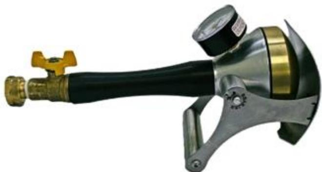
The VRI SW Spray Shower Tester IPX 3/4 is designed to perform tests in large and small scale products. It is a great option when a portable tester is necessary. It is an alternative to the Oscillating Tube for establishing the degree of protection against ingress water.
